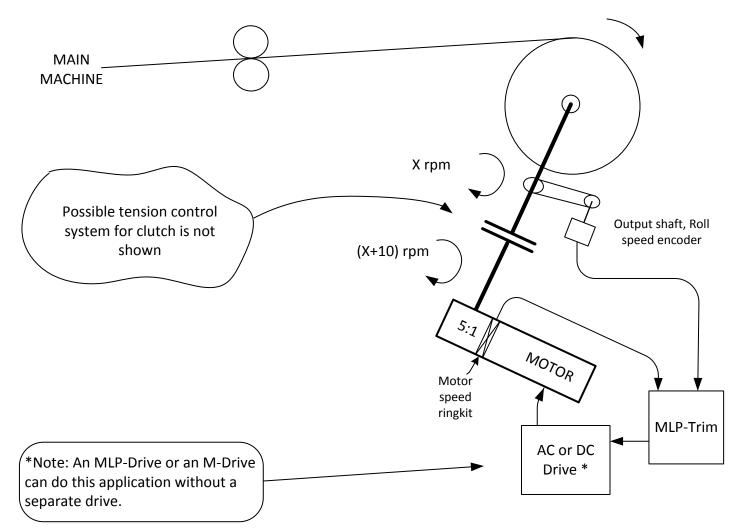
There are some applications where using a load cell or dancer is difficult or not possible. As discussed in the rest of this paper, Contrex usually controls tension directly using dancers (or load cells) and very accurately controlling the rewind speed. These systems are less expensive and do a better job of controlling tension. That said, the same precise, low-cost digital technology can optimize other technologies, like clutches and brakes.
