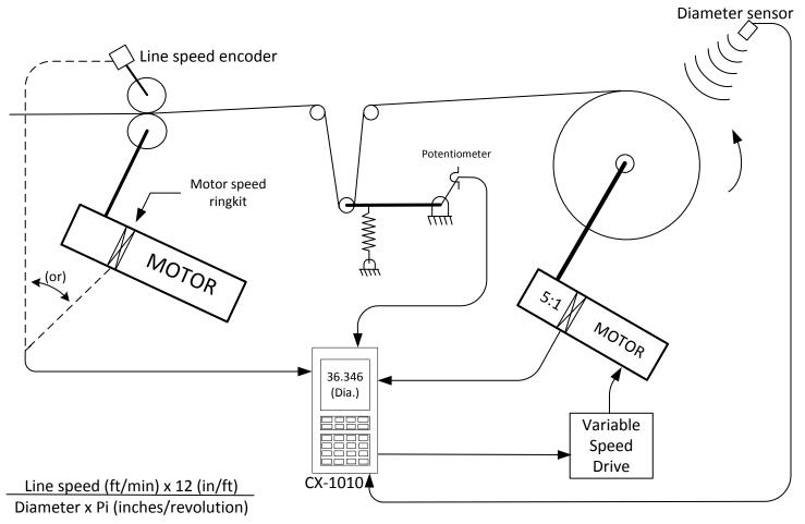
= Required revs/min of unwind roll
