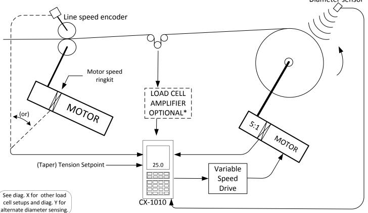
Combining the load cell system in diagram M, with the sonic system of diagram K, we get a system that does not need a reset pushbutton and can have the tension as a setpoint. Since unwinds are much more likely to have various starting sizes of rolls, this system is more likely to be used on an unwind than a winder. In both cases, the diameter information gives the CX-1010 a very precise starting point to control tension.
