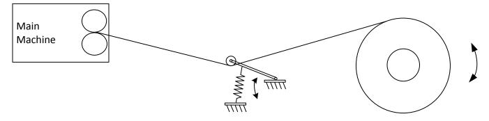
Force on the dancer could be an air cylinder, weight, or spring. The greater the amount of storage in the dancer the better. That said, a dancer with limited storage (above) will be easier to set up and tune than a typical load cell. There are many other "limited motion" dancer methods possible, besides the one shown above.
