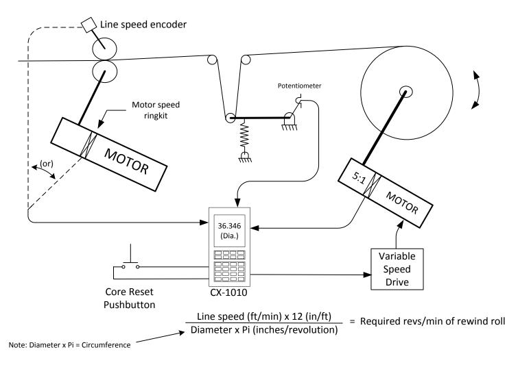
This application is similar to diagram E, with a couple of key differences. Most importantly, it does NOT require a surface speed sensor like the MLP-Trim. Using a motor sensor (like a quad ring kit) is a very nice improvement over the surface speed encoder. Besides being an expensive wear item, surface speed encoders are easily damaged and must be manually replaced by the operator, whenever the roll is changed.
