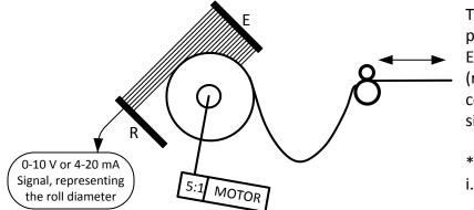
This diagram shows a opposed-mode photoelectric sensing method like the Banner EZ-ARRAY\*, which gives an analog signal (representing diameter), to the Contrex controller. The Contrex controller uses the signal as discussed in diagram K and N.
