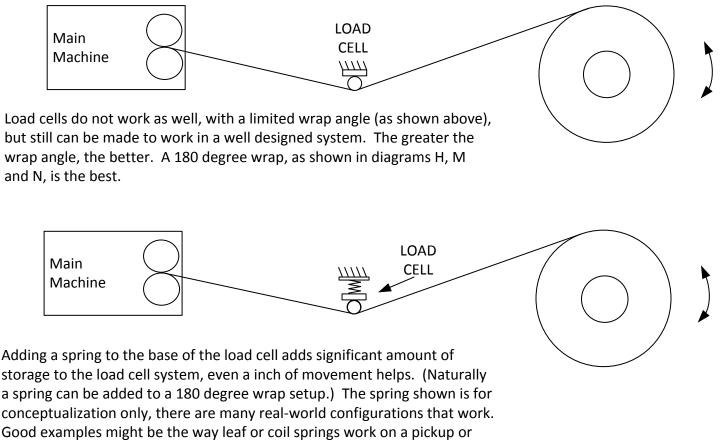
cantilevered leaf springs holding the load cells.
