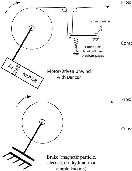
Pros: Very accurate tension No tension spike to accelerate roll No change in tension as diameter shrinks Near zero tension, as shown in diagram Y Absorbs variations from egg-shaped roll Absorbs variations from downstream machine
