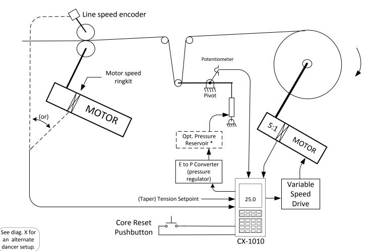
This diagram takes the set up in diagram J and adds a great way for the CX-1010 to directly control tension. After the initial speed match, the primary function of the CX-1010 is to maintain the dancer position. (Note: it is position, not tension.) A side benefit of using the CX-1010 is the ability for the operator to enter desired tension as a number, i.e. 25 lbs, instead of adjusting a potentiometer and the CX-1010 does the rest.
