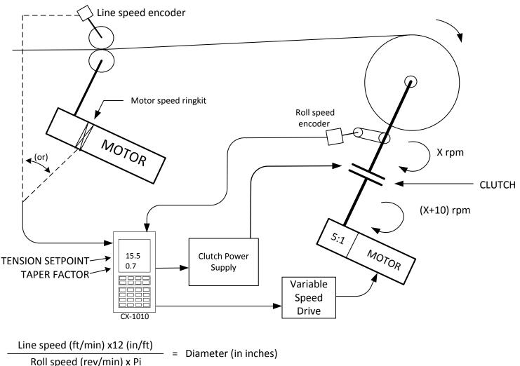
Similar to diagram U, this system does not need load cells or dancers for tension control. The math and logic of the CX-1010 can be used to optimize the performance of other technologies, or in this case perform a function that is not normally available with these traditional technologies.
